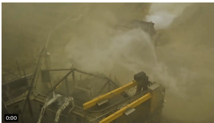
SpaceX @SpaceX · 19 mai Raptor test firing into a water cooled steel plate 🔥
